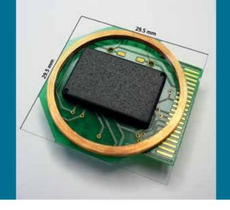
15 cm. As external components for the ASIC, only an antenna based on a coil with a resonance capacitor and an additional capacitor for smoothing the operating voltage are necessary, reducing cost and increasing reliability of the system (Figure 4). The sensor is calibrated in a fully automatic way, storing the calibration coefficients for pressure and temperature in the onchip and system EEPROM.
